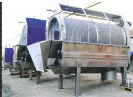
Rotary wedge wire screens with internal or external in-flow by means of drums are intended to non-pressure removal of solid particles from fluids. We offer also rotary drums based on woven screens.
