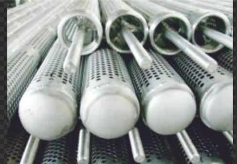
Perforated screens are applied in the washing process to remove solid impurities from product stream. They are also used as dewatering elements of beet pulp presses, and as frames for fabric bags in candle filters.
