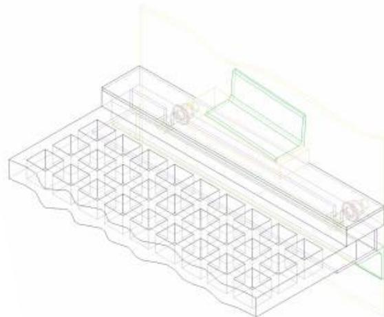
**RUBBER SCREENS WITH STEEL FRAME**, made of angle bar and steel
